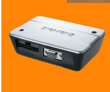
standards in the field of machine-to-machine communication. It features a Java™ software development platform, a wide range of standard interfaces plus GPRS class 12. Due to its quad-band support, the intelligent terminal can be employed in GSM and GPRS networks anywhere in the world. The integrated TCP/IP stack enables the use of IP-based services through powerful GPRS connections.
